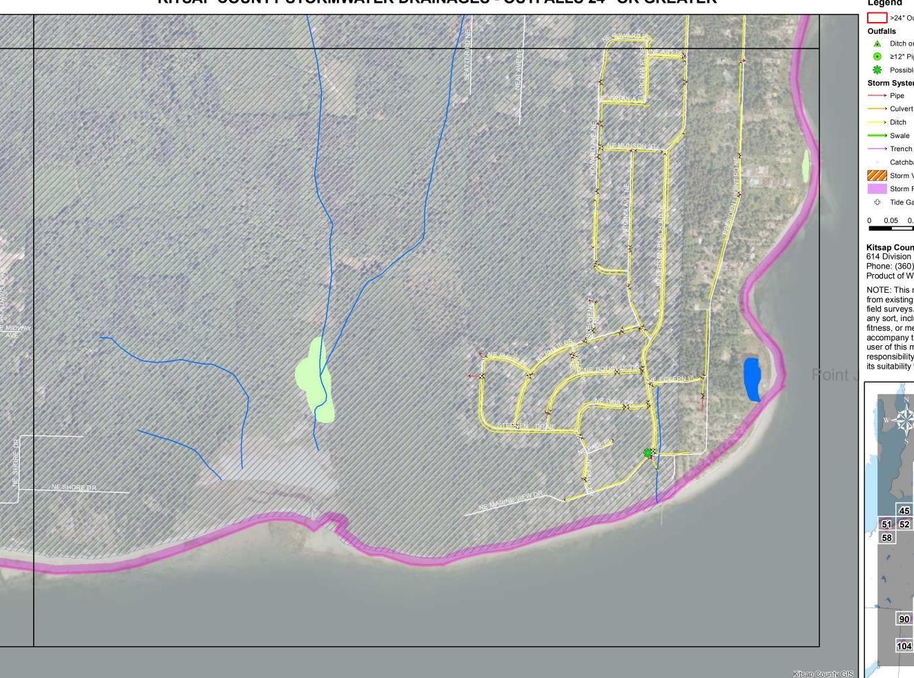
26 Legend >24" Outfall Drainage DNR Hydrology → DNR Stream Line Outfalls ▲ Ditch or Swale Island • ≥12" Pipe Lakes \* Possible New Outfall Wetlands **Street Center Lines** Storm System — Pipe Minor Road — Culvert Major Road → Ditch State Highway MS4 Area
